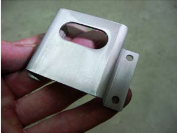
Pre-bent frame showing punched out oval, and mounting holes.
