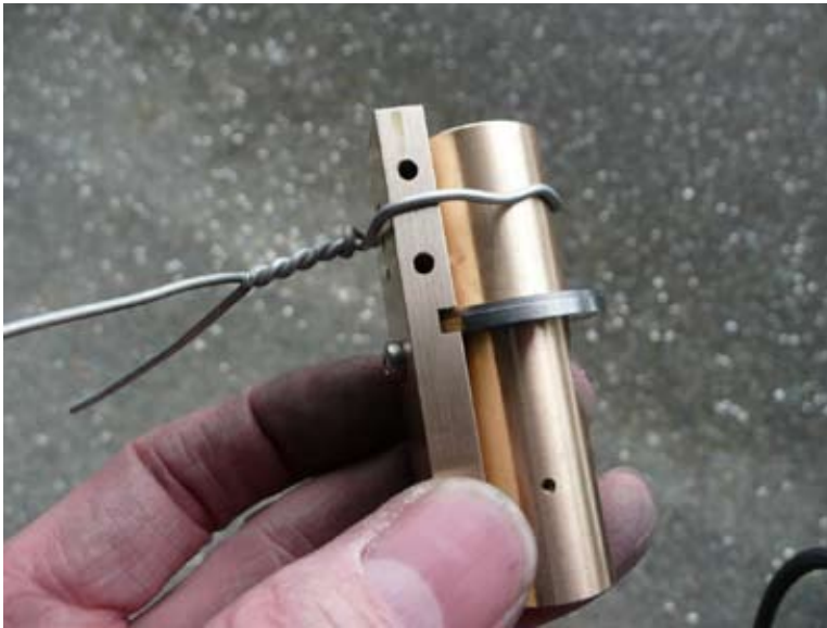
Armature wire securing frame and cylinder, ready for soldering.
