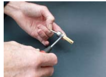
Attaching connecting rod to yoke.
