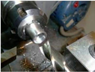
Drilling inside of trunk guide using an end mill.
