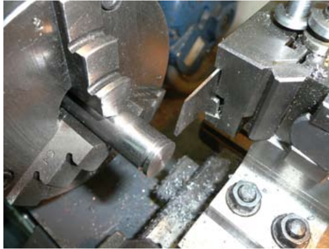
Using rear-mounted parting off tool to machine slot.
