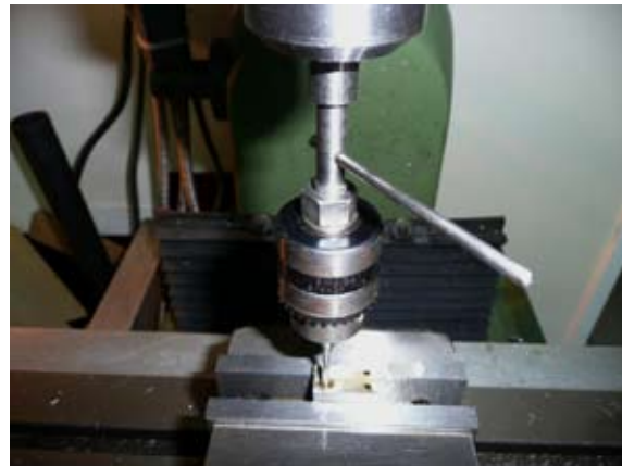
Tapping end plates in milling machine using simple tapping fixture.
