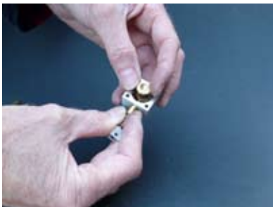
Assembling valve chest.
