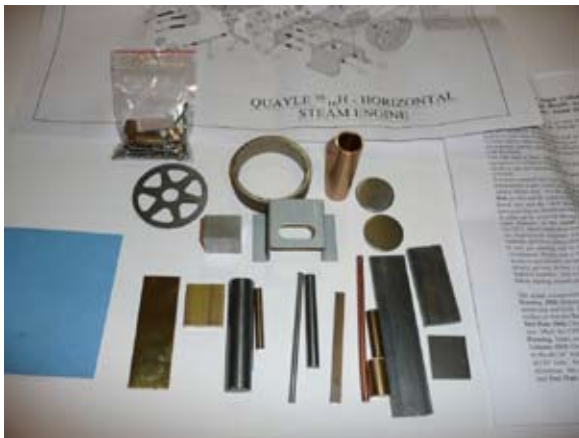
The contents of the kit - metal, plans and fittings.
