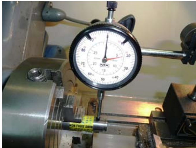
Using D.T.I to setup offset for the eccentric hole.
