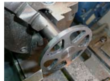
Turning outside of flywheel hub, soldered on shaft.
