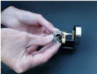
Attaching piston to shaft.
