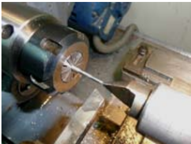
Turning down stainless steel valve rod.
