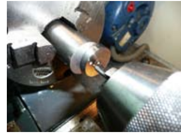
Drilling off-centre hole for crank pin in crank disk using jig.
