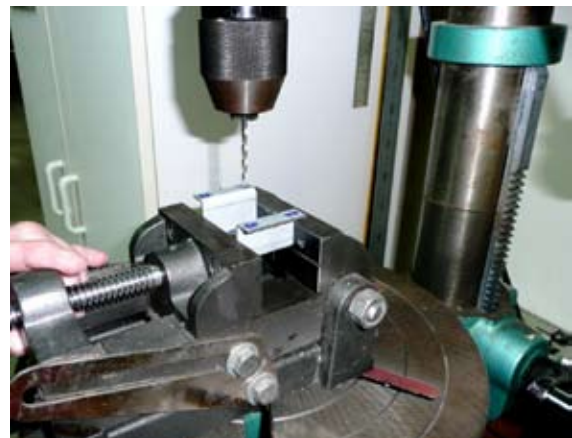
Drilling holes in the base frame.
