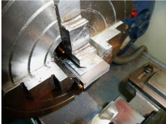
Facing off the ends of the end plates in the four jaw chuck.
