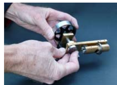
Attaching flywheel to crankshaft.
