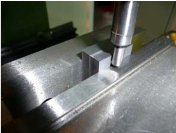
Using a "Wobbler" to find the edge of the end plates in the milling machine.
