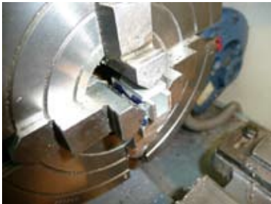
Facing off yoke in 4 jaw chuck.
