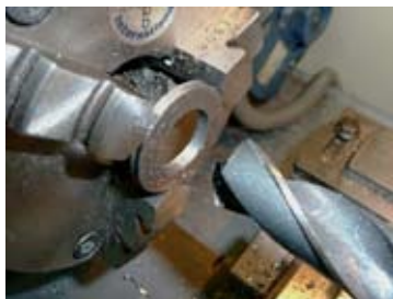
Drilling hole in lower cover.
