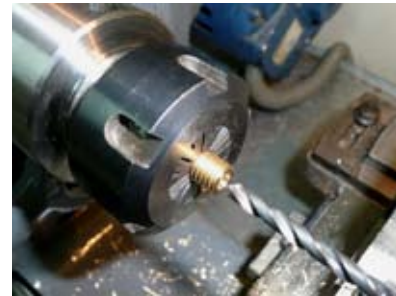
Drilling gland nut, held in a collet chuck.
