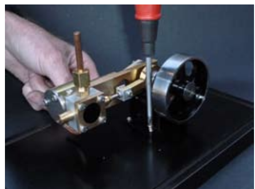
Securing Finished engine to the base.
