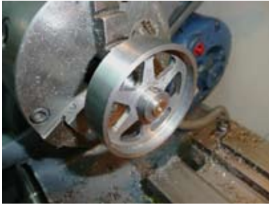
Flywheel after assembly - turning outside.
