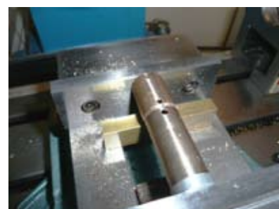
Drilling holes in the cylinder/trunk guide, starting with small holes.
