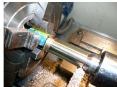
Turning the outside of the cylinder/trunk guide .
