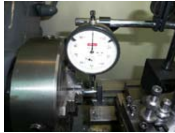
Using a D.T.I to setup offset.
