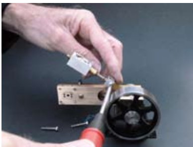
Attaching valve chest to eccentric strap.
