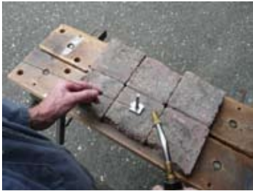
Silver soldering crank disk & crankshaft.
